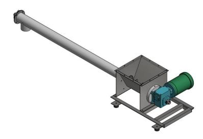
**Gearbox** lubrication is for life, as long as there are no leaks. Leaks should be addressed as soon as possible. A leaking seal is often a sign of a failed bearing.
